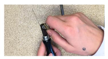
Next, tighten the saw blade. Open the screw on the back slightly, use a table and hold the back of the frame on the table while pushing downwards on the handle, once the blade is tight, tighten the screw again.
