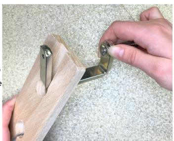
Mark on the wire, where you want to saw, with a permanent marker. Hold the saw at 90° when sawing. Start by gently running the saw down once, once you feel the saw take hold, keep running the saw up and down. The advantage of sawing the wire rather than cutting it, is that you get a straighter surface, and if you're using a wire over 2mm you avoid having to use heavy duty wire cutters.
