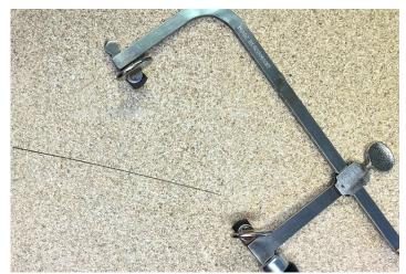
Adjust the length of the saw frame with the screw at the back, to start with, it should be set so that the blade can just fit, that way you can tighten the blade correctly. Open the screws slightly and place the saw blade between the 2 plates right by the screws and tighten them.
