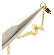
Close the jumpring again carefully with the two needle-nose pliers.
