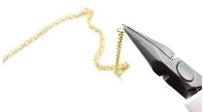
Start by opening the first jumpring with the two chain-nose pliers and pass it through the last link in the chain.
