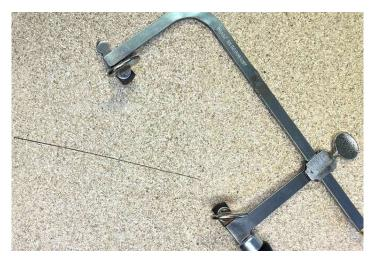
Adjust the length of the saw frame with the screw at the back, to start with, it should be set so that the blade can just fit, that way you can tighten the blade correctly. Open the screws slightly and place the saw blade between the 2 plates right by the screws and tighten them.
