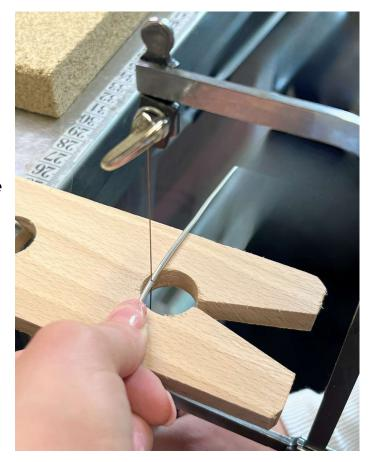
**Tip:** Always remember. If you are sawing in different directions, always remember to keep the saw in motion while changing direction. If you're in the middle of sawing and suddenly change direction without sawing, you'll realise you can't move forward and in most cases the blade will break and you'll need a new one.
