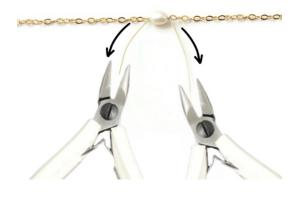
Carefully tighten the wire to close the curves.
